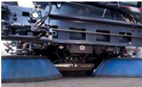
2.2 meter sweeping width with towed disc brush system & can be shifted 30 cm left & right
