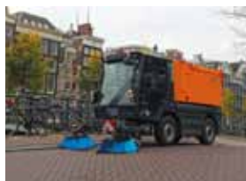
Brushes of polypropylene, steel or mixed material
